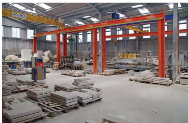
The third shed with the Gisbert totally automated ashlar flats production line in the background and finished product in foreground
